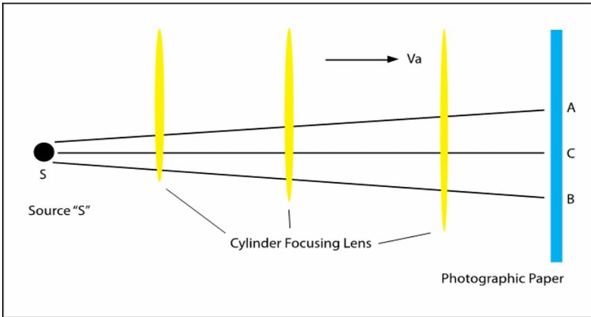
Fig. 5.5. Schematic diagram for the Proposed Experiment to detect Absolute Motion.
